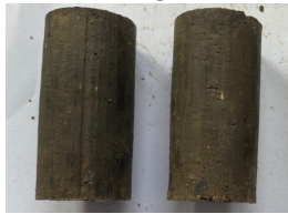
Figure 4: Properly mixed geopolymer binder and soil
