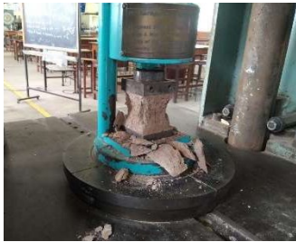
Figure 2: Compressive strength test for mortar
