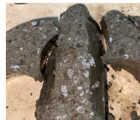
Figure 2: The flocculation of geopolymer binder before being combined with the soil
