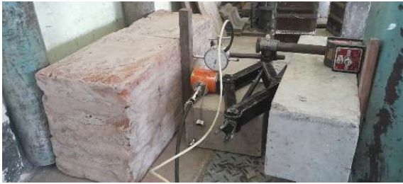
Figure 6: Out-of-plane loading test
