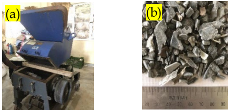
Figure 2: (a) Plastic shredder, (b) Shredded PP aggregates.
