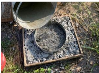
Figure 4: ASTM C1701 standard infiltration test
