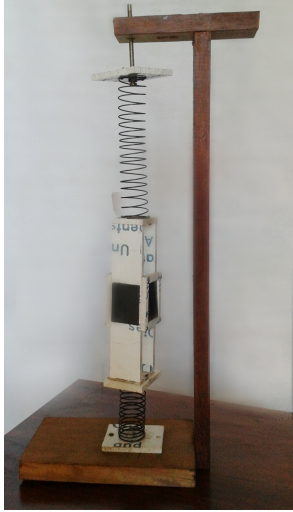
(a) Experimental setup of a SMD system (b) Experimentally measured acceleration of the SMD system.
